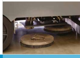
Widen the cleaning path from 1020 mm up to 1370 mm. Improve edge-cleaning and maximise productivity with an optional side brush.
